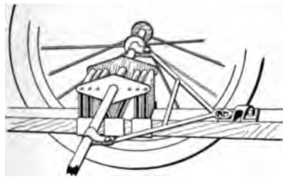
Fig. 8. Wheel Mounting Details, Wright Model B
